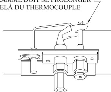
THERMOCOUPLE LA FLAMME DOIT SE PROLONGER AU-DELÀ DE LA PREMIÈRE RANGÉE DE ORIFICES.
